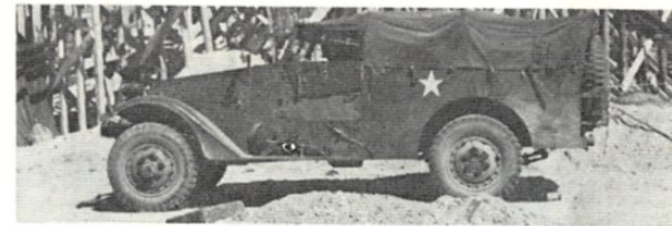
The White Scout Car with added tracks from the M2 Half-Track Truck formed the basis of the whole production series of half-tracks.
